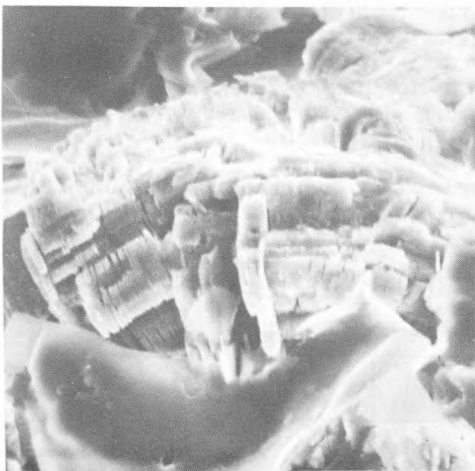
Figure 1. Kaolinite grain in RRVD 1-3, Sargent County, N.D. SEM photo 1600X.
