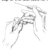
2. Sterilize the loop in the flame of the Bunsen burner. Hold the loop at a near vertical position and allow the loop most of the stem to become red hot. (Always allow the loop to cool briefly before touching bacterial broth or plate.)
